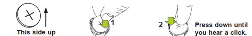
Figure 23. Install the battery
